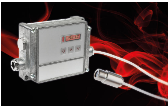
The measuring head of the OI98C558 can be used at ambient temperatures of up to +180°C. The system solution including evaluation unit is particularly suitable for contactless temperature measurement of objects with high heat radiation. (all images: ipf electronic gmbh)
